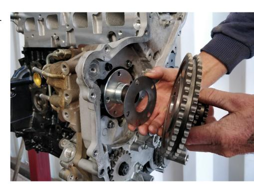
Using a straight edge on the vacuum pump sprocket check the fuel pump alignment with the vacuum pump sprocket. There is end float in both pump shafts. The fuel pump sprocket must be in alignment with the vacuum pump sprocket. The factory does not always fit the correct shim. Shims are .50, 1.0, 1.2, 1.6. To achieve exact alignment of the fuel pump sprocket surface linish the mounting face of the fuel pump sprocket. To see how this is done go to yd25.com.au information video page
