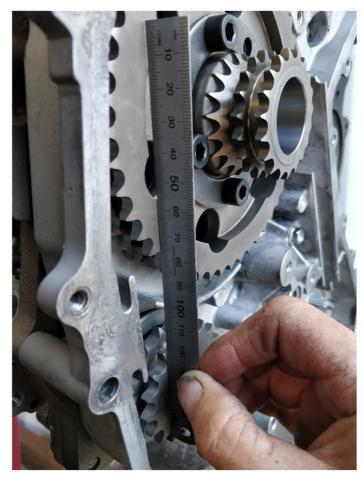
Check alignment between fuel pump sprocket and crankshaft sprocket. If the alignment adjustments were done correctly these sprockets will be in alignment.
