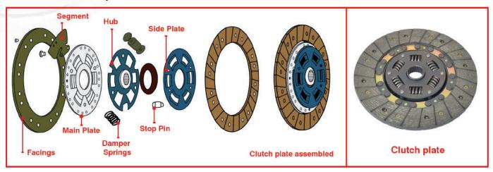
Around the outside of the clutch plate, on both sides, there is a hoop of friction material. The friction material riveted to the disc is designed to grip the flywheel. Because of the interlocking spline, the clutch plate and gearbox input shaft will then turn together.
