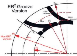
radius increases so does the Torque Capacity of the clutch. This system can be found in both the Mantic and 4Terrain performance clutch range.
